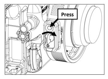
4. Press and hold the port release safety button, turn the port lock/release latch clockwise until it stops.
