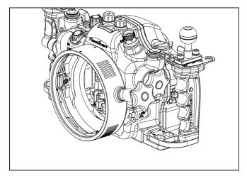
Install the camera body only into the housing and mount the adaptor to the housing.
