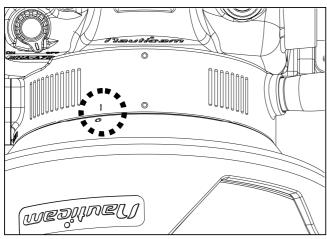
5. Align the "I" mark on the adaptor with the WHITE dot on the port. Gently push the extension ring towards the port until it cannot go in any further.
