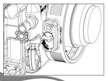
3. Lift the Port lock/ release latch on the other side of the adaptor.
