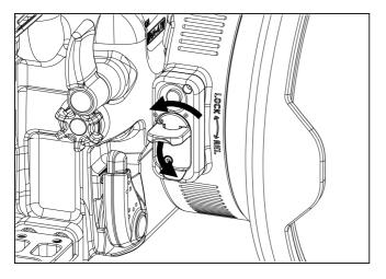
7. To lock the port in place, turn the port lock/release latch anti-clockwise to the original position and then flip it down.
