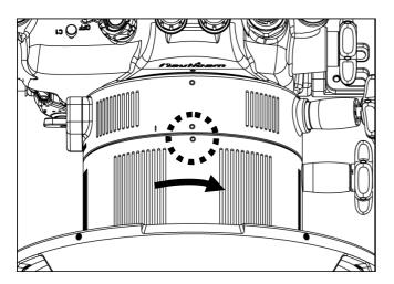
6. Turn the port clockwise until the white dot on the adaptor aligns with the white dot on the port.
